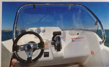
CONSOLE: The wheel is placed close to the centre line to keep the lateral weight distribution even.
